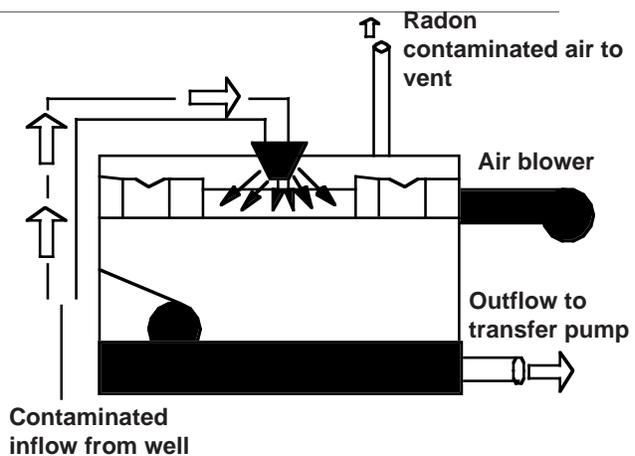
Figure 4: Radon removal by horizontally extended shallow aeration.
