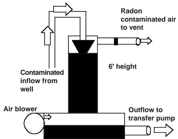
Figure 3: Radon removal with a packed column.
