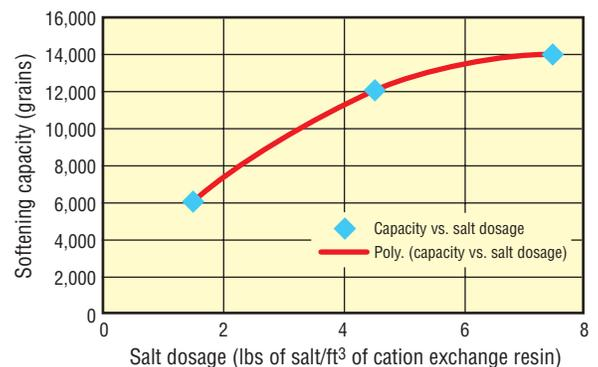
**Figure 2: Softening efficiency as a function of salt setting**
