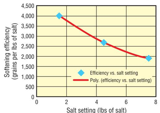
**Figure 3: NSF/ANSI 44 efficiency requirements (DIR softeners only)**
