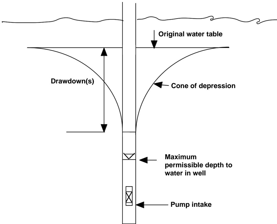
Figure 2. Well hydraulics.
