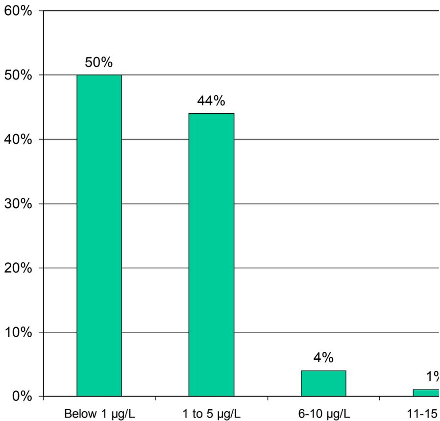
Figure 1. The frequency of occurrence of various arsenic concentrations in 578 wells in Pennsylvania (source: U.S. Geological Survey).
